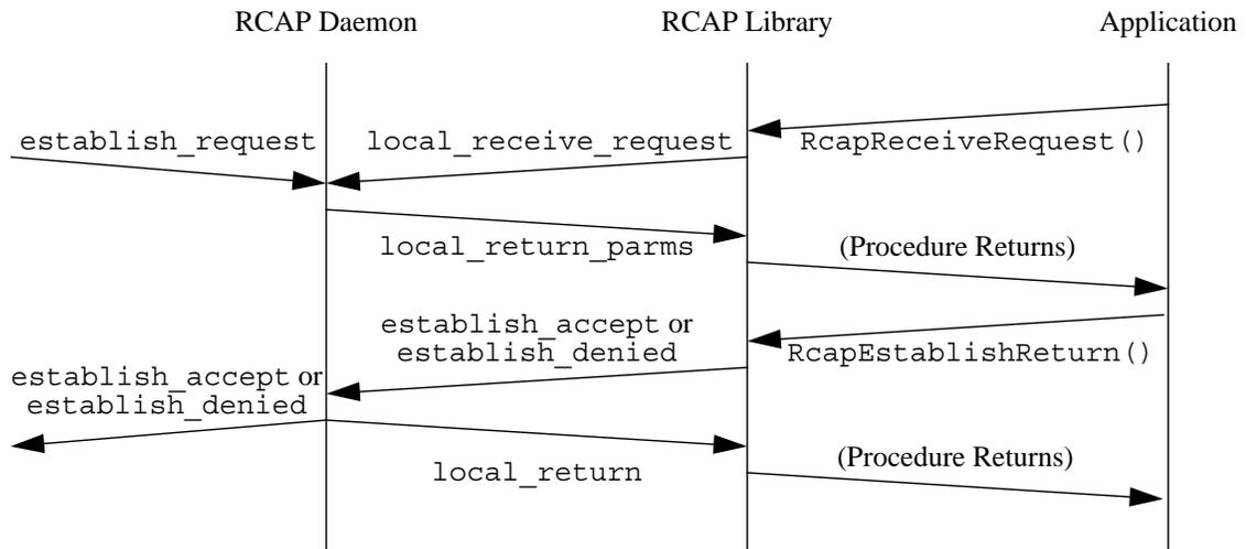
**FIGURE 5. Channel Establishment (Receiving End)**
