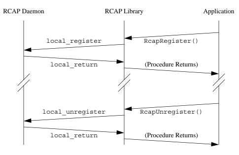
FIGURE 4. Registering and Unregistering a Receiving Application
