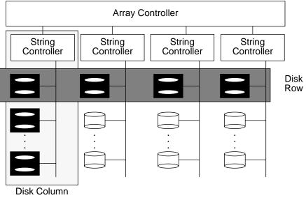
FIGURE 2. Architecture of a RAID.
