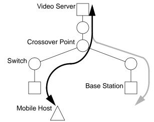
FIGURE 3. The MH has just moved from the right BS to the left BS. The existing network connection has been incrementally re-established from the crossover point.
