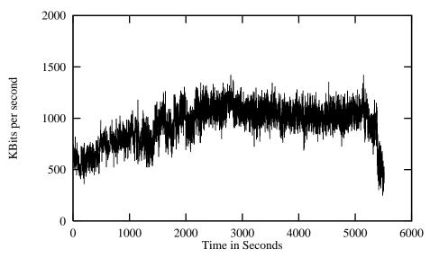
FIGURE 3. Total IP Multicast Bitrate During XUNET Videoconference, 22 September 1993.
