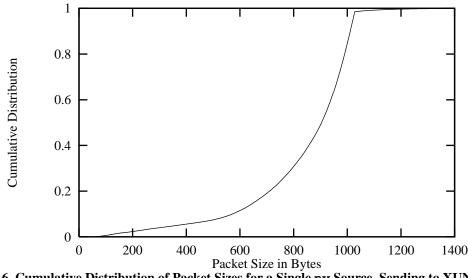
FIGURE 6. Cumulative Distribution of Packet Sizes for a Single nv Source, Sending to XUNET Video, 22 September 1993.
