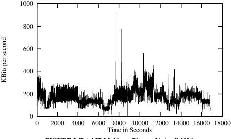
FIGURE 2. Total IP Multicast Bitrate, 21 April 1994.
