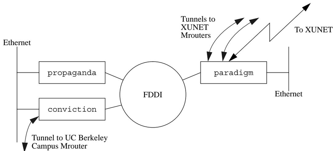
**FIGURE 1. Network Environment.** *conviction* and *paradigm* are MBONE routers; each forwards packets between its tunnel(s), its attached Ethernet, and the FDDI network. *propaganda*, the tracing host, sees all multicast traffic passing between the two MBONE routers across the FDDI network.
