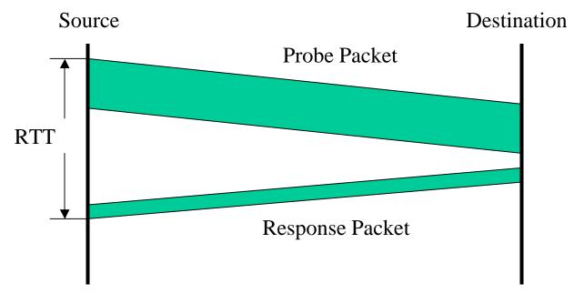
• Vary probe packet size, determine response time as a function of probe size
