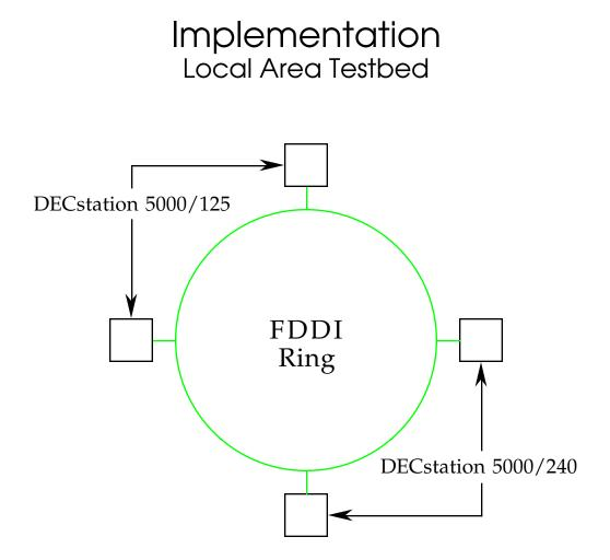
A simple environment for testing a prototype implementation.
